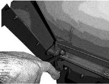
You will need to use (2) two 9/16" hex wrench. First loosen top bolts that are fastening the front cover against the Top Hopper and cutting chamber. Repeat for bolts below.
