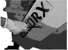
Loosen the bolt in the belt guard, and also loosen up a bolt that is located down below. Retire the cover and also make sure to take off the cover's axial support pipe (see Parts List section) and screw bar. You can do that by inserting your hand in the chamber and pulling in the screw bar.
