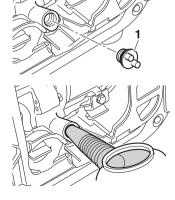
**5.** Fill the specified amount of the recommended engine oil, and then install and tighten the oil filler cap.
