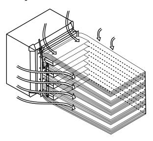
The Air Flow Induction Optimizer increases the throw for Reznor Models WS. This increased flow results in energy savings and better environmental control. This option increases the air speed thanks to the unique shape of the deflecting louvers which create layers of hot air at the unit outlet.
