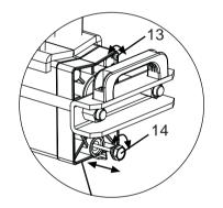
Before operating the log splitter, the Bleed Screw should be loosened by some rotations until air can go in and out of the oil tank smoothly.
