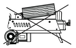
Break log in the direction of its growing grain. Do not place log across the log splitter for splitting. It may be dangerous and may seriously damage the machine.
