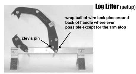
1) Attach arm and support as in photo with pins. Use clevis pin in second set of holes in arm to help crate space between support and arm. This make it easier to put the lifter over the log.
