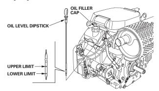
Oil is added to the engine by removing the oil cap and adding oil at this point. After filling the crankcase to the proper level, be sure you properly tighten the oil fill cap.
