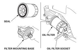
**NOTE:** This engine requires 57 to 58 ounces (1.78 to 1.81 quarts) of oil if it is completely drained. Use caution when refilling the engine as some residual oil may have remained in the engine. Always use the dipstick when filling the engine with oil to prevent overfilling.
