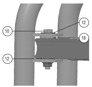
• When completed, your handles should look like this. Part 5 is installed on the back hole of the bracket with the clip facing out. Part 4 is installed on the front hole of the bracket. Either handle can go in either bracket.
