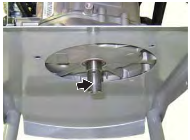
Figure 57 – Key and Crankshaft Keyway
