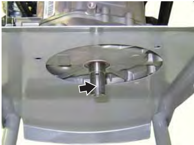
Figure 55 – Key and Crankshaft Keyway
