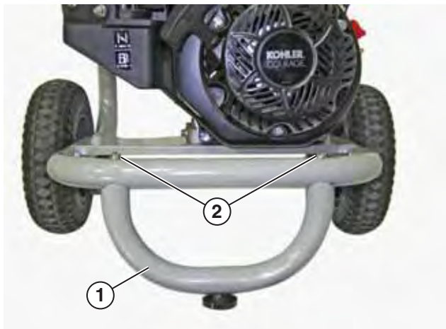
Figure 10 – Installing Front Support
