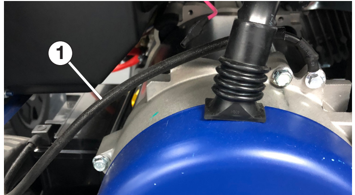
Figure 5 - Locating Negative (-) Cable
