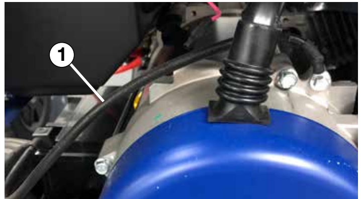
Figure 5 - Locating Negative (-) Cable
