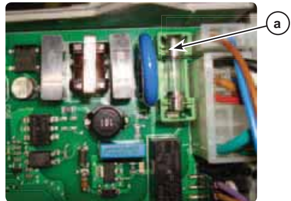
Figure 109 Thermostat-relay circuit fuse location
