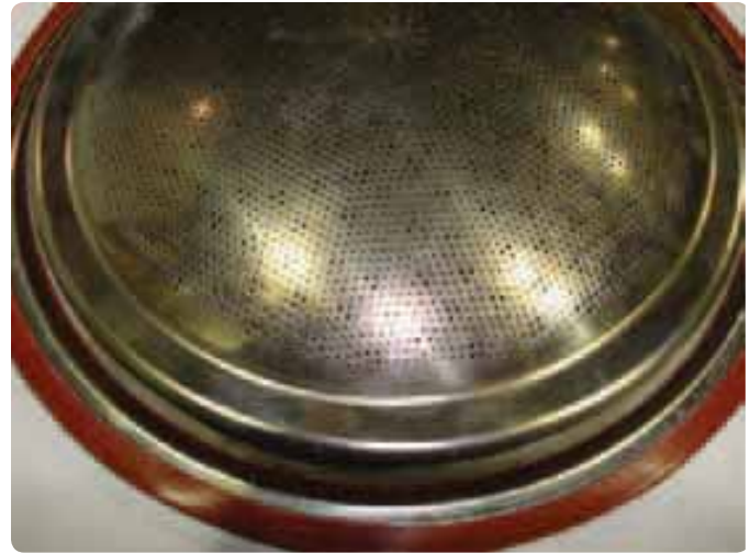
Figure 141 Inspecting exterior and cleaning the burner
