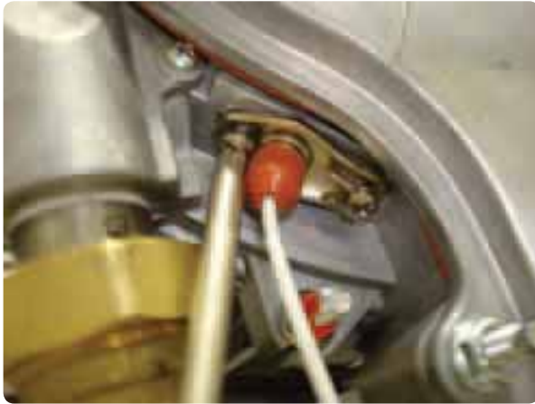
Figure 135 Removal of Ignition electrode
