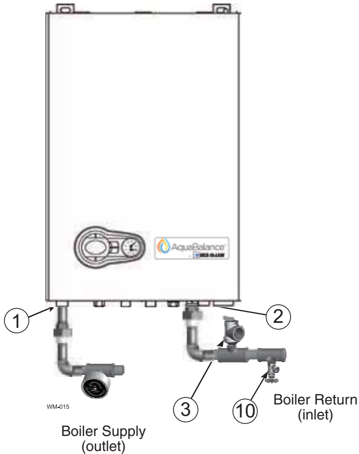
Figure 6 Install pipe fittings for relief valve and pressure/temperature gauge — DO NOT mount relief valve until AFTER hydrostatic testing (see legend below)
