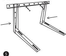
Position arms to accomodate equipment measurments and tighten set screws. Use remaining lag screws or anchors to secure bracket arms.
