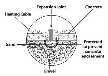
ProMelt must be embedded in a sand bed when transitioning out of the concrete slab.
