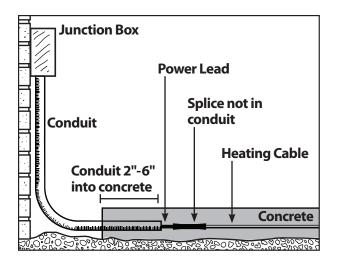
ProMelt electrical leads transition from the slab to the control or electrical junction box via conduit.
