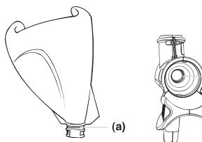
After all components are clean, wipe down with a dry cloth. Reassemble the sprayer/turbine. ON/OFF switch should be facing upward. Clean turbine labels with a damp cloth.
