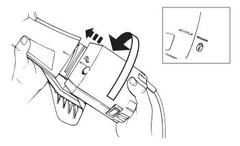
While facing the rear of the sprayer/ turbine assembly, insert the hopper into the receptacle with the hopper oriented as shown. Depending on what surface you plan to spray, turn the hopper 1/4 turn in either direction to lock it in place.
