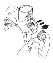
4. The nozzle, sprayer and the hopper can now be hand-cleaned using warm, soapy water and the cleaning brush provided with the unit. Let faucet water run into the area where the hopper connects to the sprayer. While the water is running, activate the trigger to fully clean the nozzle area . DO NOT sumberge the turbine. The outside of the turbine can be wiped clean with a damp cloth.
