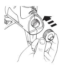
4. Slowly fill the hopper with the material you plan to use. Be sure the sprayer/ turbine assembly is resting on a flat, stable surface that is covered by a drop cloth.
