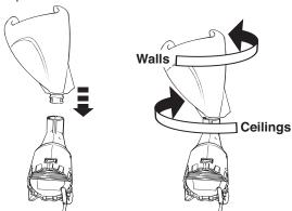
Attach desired nozzle by threading it onto the end of the sprayer.
