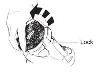
While pressing the disc lock on the bottom of the unit, thread new disc onto unit by turning it clockwise and tightening by hand.
