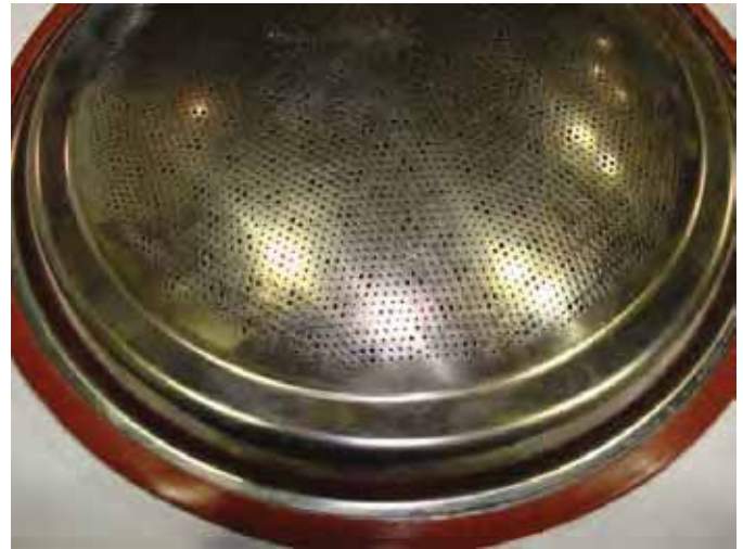
Figure 135 Inspecting exterior and cleaning the burner
