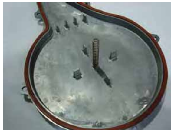
Figure 132 Heat exchanger cover plate removed
