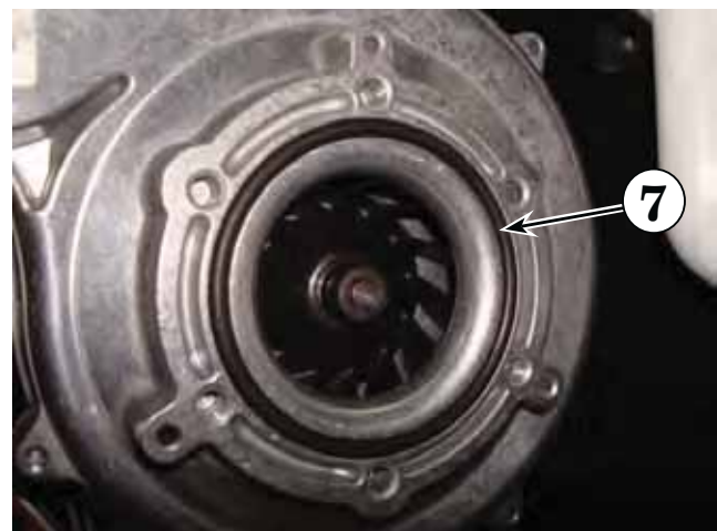
Figure 16 Insure "O" ring is in place.
