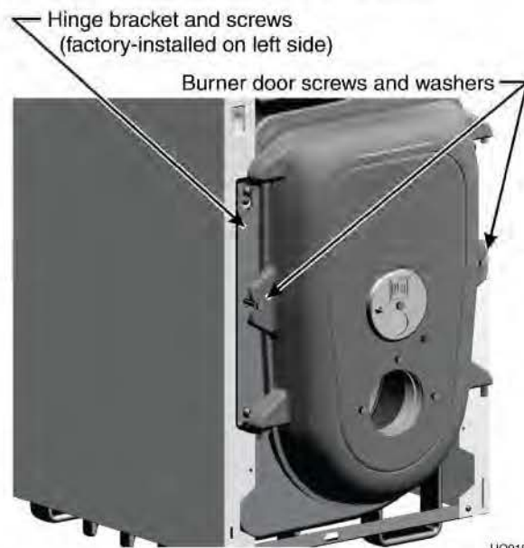
Figure 4 Burner door hinge installation
