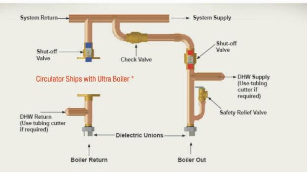
\* Circulator is not included in the Ultra Easy-Up Manifold Kit, a circulator ships with every Ultra boiler
