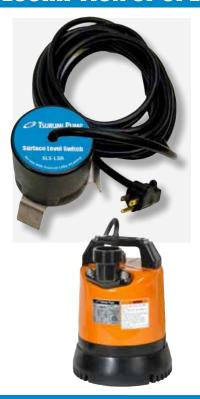
The Surface Level Switch with Lift Bracket is used to automate a utility/ floor sucking pump. Set the Surface Level Switch on the floor and plug the power cord from the pump into the piggyback plug on the switch. Plug the piggyback plug into a standard 120 VAC wall outlet (the unit will also work on GFI outlets).
