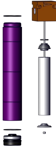
Figure #2: Oil Coalescing Filter
