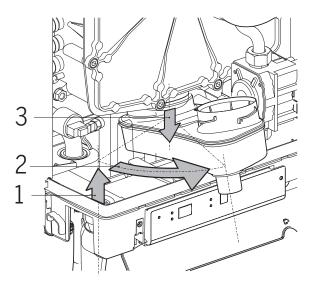
Fig. 25: Removal of Condensate Pan
