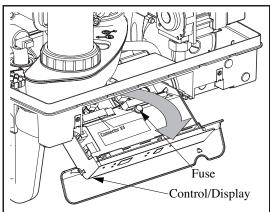
Fig. 17: Accessing Low Voltage X4 Connections
