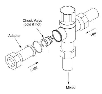
**Figure 9: Mixing Valve Assembly**
