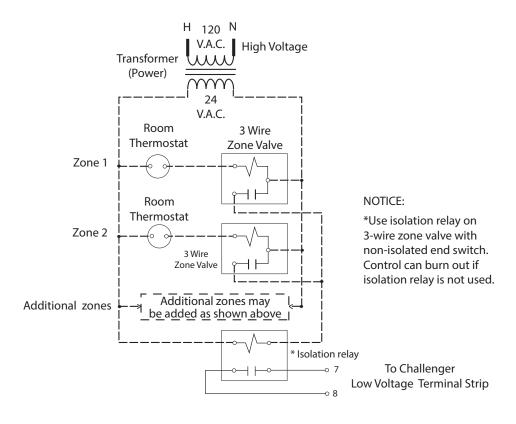
Fig. 19: Multiple Zone Field Wiring Using Zone Valves
