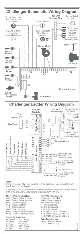
Fig. 16: CHALLENGER Factory Wiring Diagram
