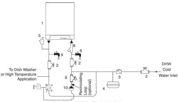
Figure 11 Domestic Piping - Standard Installations
