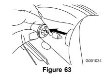
4. Insert a new bulb into the back of the headlight (Figure 64).
