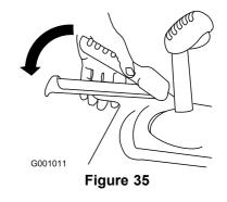
2. To stop the traction drive, release the traction lever.
