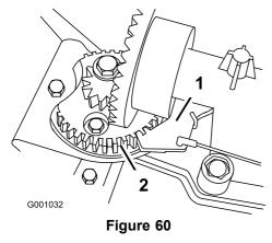
1. Discharge chute latch 2. Gear teeth
