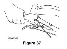
Momentarily squeezing and releasing the left or right wheel clutch lever also allows for steering adjustments to keep the machine going in a straight line, especially in deep snow.
