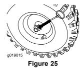
To self-propel, insert the axle pins through the holes in the wheel hubs and the inner axle holes (Figure 26).
