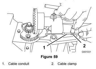
3. Grasp the cable conduit and move it toward the front of the machine until the discharge chute latch fully engages the gear teeth (Figure 59 and Figure 60).
