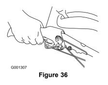
**Note:** This disengages the drive to the right wheel while the left wheel continues driving, and the machine turns to the right.
