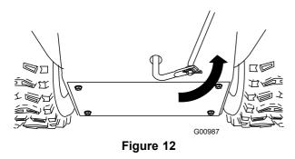
6. Lift up on the speed control rod and insert the trunnion into the hole in the speed selector lever (Figure 11).
