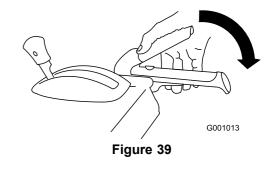
To stop the auger and impeller, release the right hand 2. lever.
