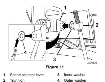
**Note:** To make installation easier, leave the flat washer on the trunnion (Figure 11).
