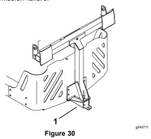
1. Bagger support bracket with drawbar
