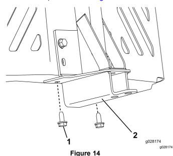
1. Self-tapping screw (5/16 x 2. Pivot frame 3/4 inch)
