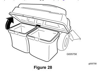
Compress debris into the bags. With both hands, lift up on the bag and unhook it from the
