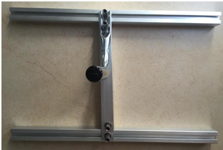
4. Attach shield (#20) to the long rails (#7) using bolts (#18), washers (#11), and nuts (#4).
