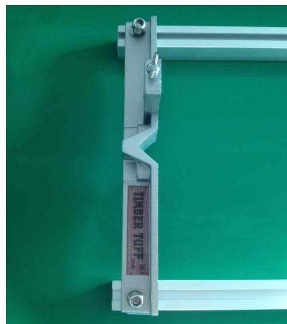
7. Attach chain guard assembly to the frame bracket (#6) using U-Bolt (#9)m U-Bolt Adaptor/Clamp (#10), washers (#11), and long hex nuts (#2).
