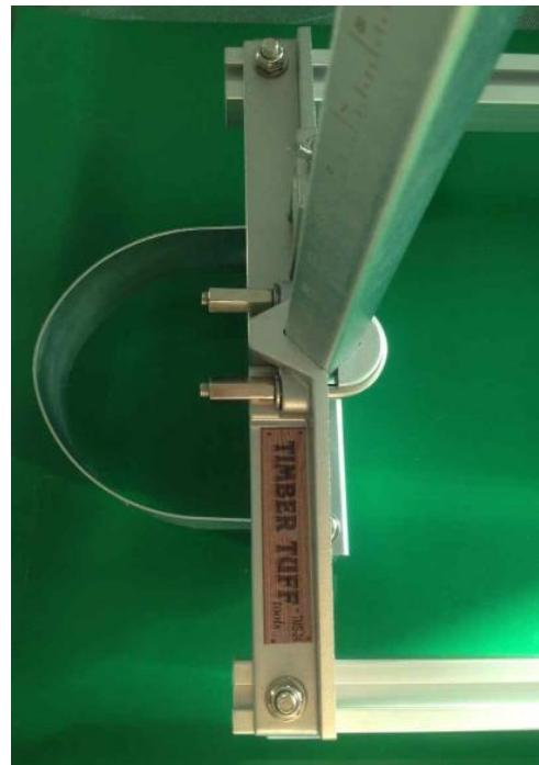
With the guard assembly attached to the frame bracket and long rails, adjust to desired cutting thickness (minimum 3 inches) and tighten nuts around U-Bolt.
