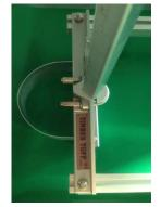
With the guard assembly attached to the frame bracket and long rails, adjust to desired cutting thickness and tighten nuts around U-Bolt.
