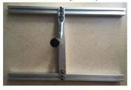
4. Attach shield (#20) to the long rails (#7) using bolts (#18), washers (#11), and nuts (#4).
