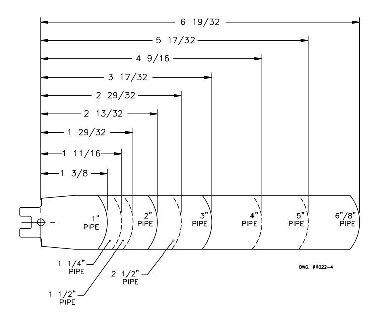
Flexible paddles smaller than the actual pipe size should be used for added support and higher sensitivity. See Fig. 2. The paddles must be properly attached and the screw that holds the paddle must be securely tightened.
