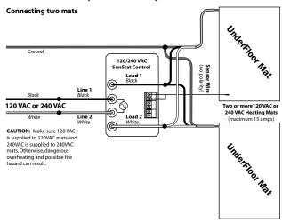
All electrical work must be done by a qualified, licensed electrician in accordance with local building and electrical codes, and the National Electrical Code (NEC), especially Article 424, Part IX of the NEC, ANSI/NFPA 70 and Section 62 of CEC Part I.
