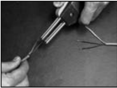
Step 2.7. Use thermal wire strippers to remove ½" of the insulation from the heating wires.
