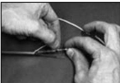
Step 2.11. Slide a solder tube over a heating wire. Place the heating wire and jumper alongside each other. Lightly twist their stripped ends together to help join them in a "Western Union splice" technique.
