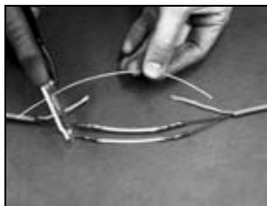
Step 2.15. Cut a bare jumper wire shorter, if necessary, so that it overlaps the braid shield pigtail by at least 1/2" on each end.
