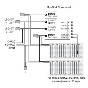
Electrical Wiring Diagram for SunStat Command with SunStat Relay C3 (120/240 VAC). Up to 10 SunStat Relay C3's can be connected to expand the area controlled by a single SunStat Command.
