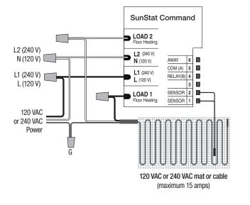
Typical Wiring for SunStat Command with multiple mats or cables (120/240 VAC).
