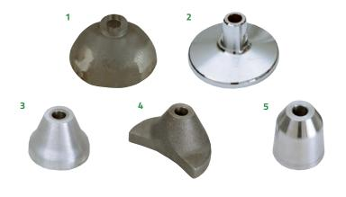
Backfill Tamper Butts, like all Sullair accessories, are made specifically for Sullair tools, so proper fit and performance are assured. Our selection includes: (1) 6" Malleable Iron, (2) 6" Steel Butt (standard), (3) 4" Aluminum Butt, (4) Pole Butt Half Moon and (5) 3" Aluminum Butt.
