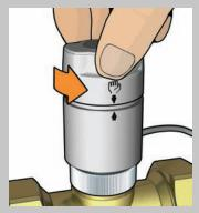
When power is interrupted or when you need to check the operation of the actuator, you can manually open it with a twist of the top.
