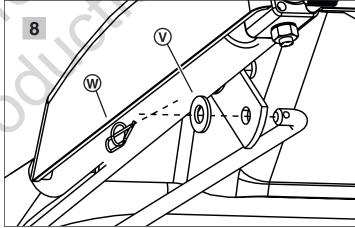
9. Tighten the hex nut against the ball joint.
