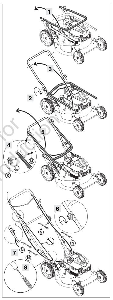
9. Using the fifth cable tie (N), secure the engine speed control cable to the oil fill tube on the right rear of the engine.
