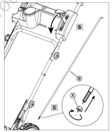
7. Thread the ground speed rod into the ball joint on the speed control pivot arm until the elbow on top of the ground speed rod is lined up with the hole in the bottom of the ground speed lever (inset).
