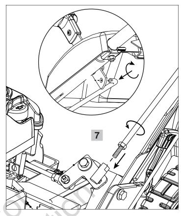
Insert the ground speed rod into the ground speed lever.
