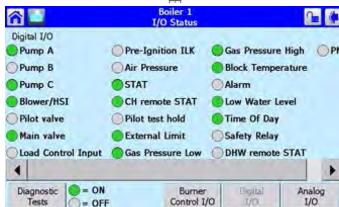
Figure 69 Digital I/O Status page (HOME PAGE → → DIAGNOSTICS)
