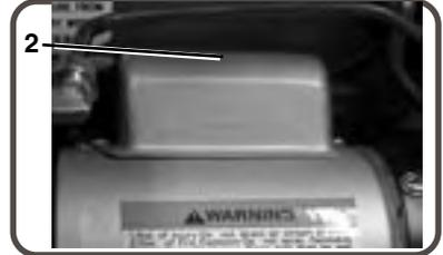
**3) AIR INTAKE FILTER:** This filter is designed to clean air coming into the pump. To ensure the pump continually receives a clean, cool, dry air supply this filter must always be clean and ventilation opening free from obstructions. The filter can be removed for cleaning by using warm, soapy water. Rinse the filter and air dry.
