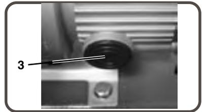
**4) AIR COMPRESSOR PUMP:** To compress air, the piston moves up and down in the cylinder. On the downstroke, air is drawn in through the air intake valve while the exhaust valve remains closed. On the upstroke, air is compressed, the intake valve closes and compressed air is forced out through the exhaust valve, into the discharge line, through the check valve and into the air tank.
