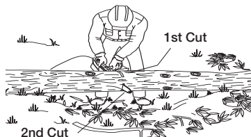
Figure 16 - Bucking Log When Log Is Supported On Both Ends
