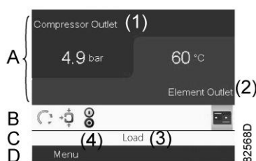
Typical Main screen (2 value lines), fixed speed compressors
