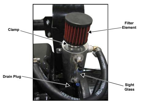
Figure 5-15. Drain Breather Canister and Replace Filter
