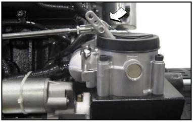
Figure 5-16. Lubricate Governor Rod Ends
