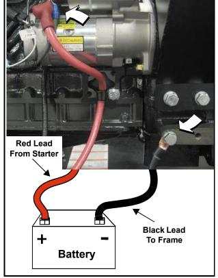
Figure 5-11. Battery Cable Connections
