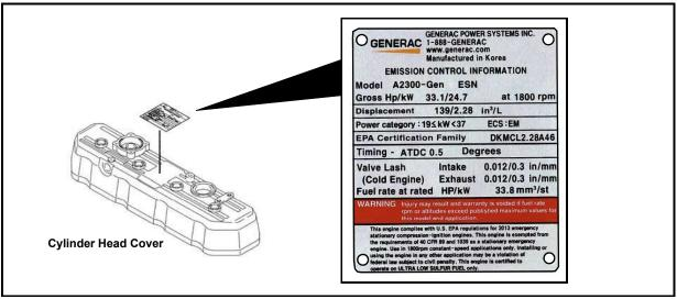
Figure 2-1. Emissions Data Plate (Sample)
