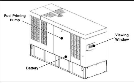
Figure 3-1. Enclosure (Rear Left View)
