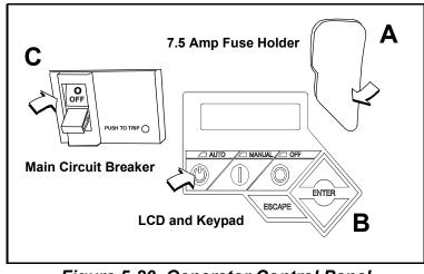
Figure 5-20. Generator Control Panel
