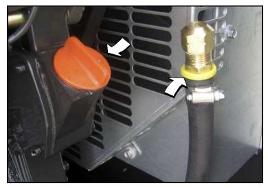
Figure 5-17. Oil Fill Cap and Drain Hose
