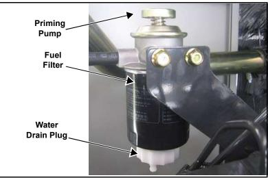
Figure 5-8. Drain Water From Fuel Filter
