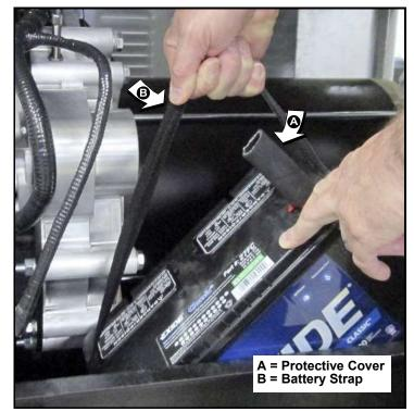
Figure 5-12. Install Battery (2.3L Models)
