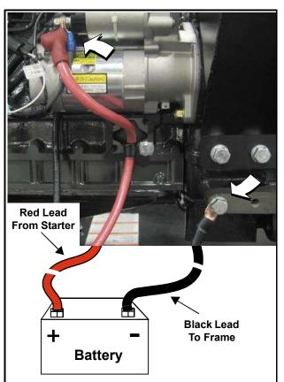
Figure 3-4. Battery Cable Connections
