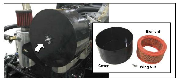
Figure 5-14. Air Cleaner Cover and Filter Element
