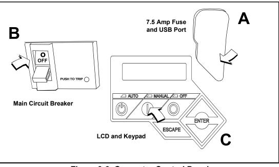
Figure 3-6. Generator Control Panel
