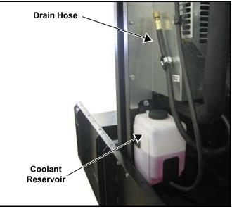
Figure 5-9. Coolant Overflow Reservoir and Drain Hose
