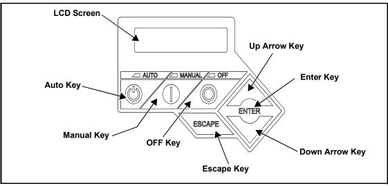
Figure 4-2. Control Panel Keypad and LCD Screen
