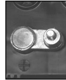
POSITIVE POST HAS LARGER DIAMETER
