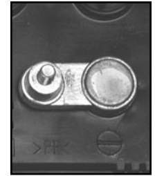
NEGATIVE POST HAS SMALLER DIAMETER
