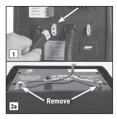
battery—the BLACK wire to the POSITIVE (+) post and then the WHITE wire to the NEGATIVE (-) post. Tighten the bolts on the battery posts. (e) Plug the control unit back into the wall outlet.
