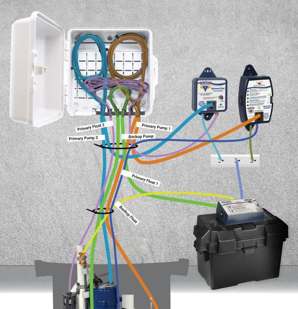
These cords typically are black. To make it easier to track which cord connects to each pump, controller or float switch, every cord is depicted in a unique color.
