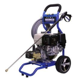
Engine Brand: Honda GX390 Starter: Recoil **CC:** 389cc Oil Alert: Yes Oil Type-Engine: SAE 10W30 Fuel Tank Size: 6.4 U.S. gts Pump Brand: Terminator Pump **Pump Type:** TC3-13X13.0 Oil Type-Pump: SAE 15W40 (Sealed) Adjustable Pressure: Yes Chemical Injection: Down stream injection Water Temperature: 50°C/120°F Water Pressure: 4200 PSI Water Flow: 4.0 GPM Frame Type: Large cart Wheels: Flat free
