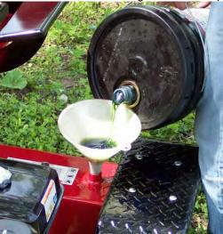
NOTE: The total hydraulic system oil capacity for this unit is approximately 10 gallons.
