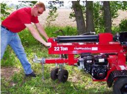
2. Make sure both ends of the log you are splitting are cut as square as possible. This will prevent the log from sliding out of position while under pressure. All logs should be 24 inches long or shorter.
