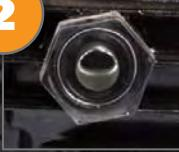
Fill pump with SAE 30 (non detergent) oil until filled half way through the sight glass.
