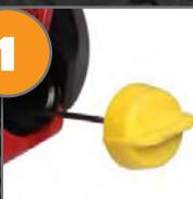
Fill crank case with 10w30 weight oil until oil is visible at the top of the dipstick.
