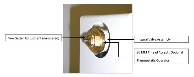
Flow Setter is adjusted by turning the inner gland (picture above) to the corresponding number.
