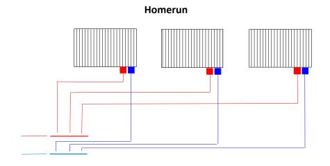
Homerun with Thermostatic Operators and By-Pass Valve
