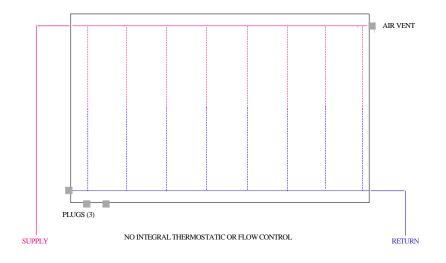
PENSOTTI PANEL RADIATORS - ALTERNATE PIPING ARRANGMENT 1
