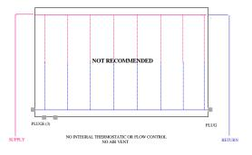
PENSOTTI PANEL RADIATORS - ALTERNATE PIPING ARRANGEMENT 4
