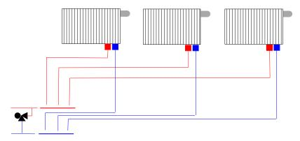
Homerun with Electric Zone Valve and By-Pass Valve
