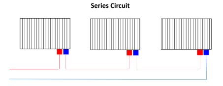
Series Circuit w/ By-Pass Valves (Maximum Circuit Flow Rate Is 2 GPM, And / Or 4 Radiators)
