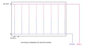
PENSOTTI PANEL RADIATORS - ALTERNATE PIPING ARRANGEMENT 7
