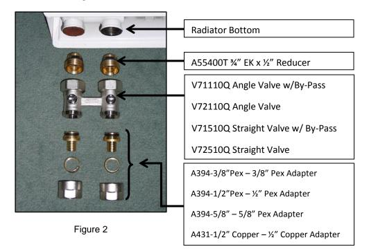
**Figure 1 Pex**: Insert the A55400T reducers into the supply and return connections of the radiator and tighten with a 12mm allen wrench. Choose the proper size pex tubing adapter assembly, slide the nut
