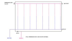
PENSOTTI PANEL RADIATORS - ALTERNATE PIPING ARRANGEMENT 5
