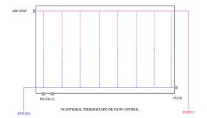
PENSOTTI PANEL RADIATORS - ALTERNATE PIPING ARRANGEMENT 2
