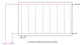
PENSOTTI PANEL RADIATORS - ALTERNATE PIPING ARRANGEMENT 6
