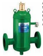
Air separator. Epoxy resin coated steel body. 1 NP bottom thread. ANSI flanged connections. Max. working pressure: 150 psi. Working temperature range: 250°F. ASME National Board egistered
