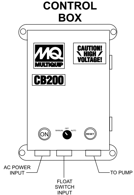
Figure 3. Electrical Control Box (CB200)
