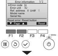
Error code, error unit, refrigerant address, unit model name, and serial number will appear.
