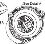
30 Functionally check the lower guard with the saw set at full depth of cut and zero degree bevel. Place the saw upside down with the shoe horizontal. Retract the lower guard 100%. Release the lower guard lever. The guard should return in a brisk manner.
