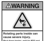
Shut down tractor, wait for PTO and all moving parts to come to a complete stop, then disconnect PTO shaft from tractor before opening.
