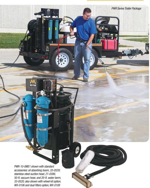
The PWR Series allows for wash water to be reclaimed on the jobsite. Water is reclaimed by using the 20-foot water berm (included) to stop water from flowing down a drain or away from your area. The suction head draws wash water into a holding chamber where a second pump forces the water through an optional 10-micron bag filter before returning it to the holding tank for reuse or proper disposal.
