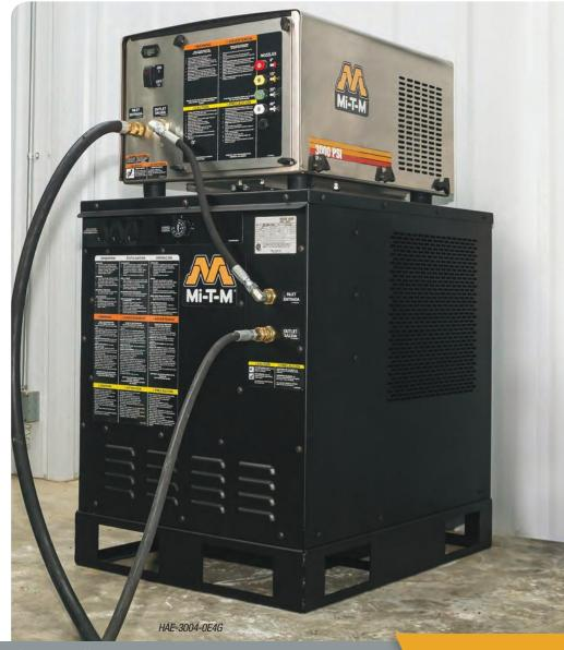
The all-electric HAE Series offers a fast and effective cleaning method without the emission of fuel and exhaust fumes. A revolutionary heat exchange cartridge design provides consistent on-demand hot water perfect for cleaning food and beverage facilities.
